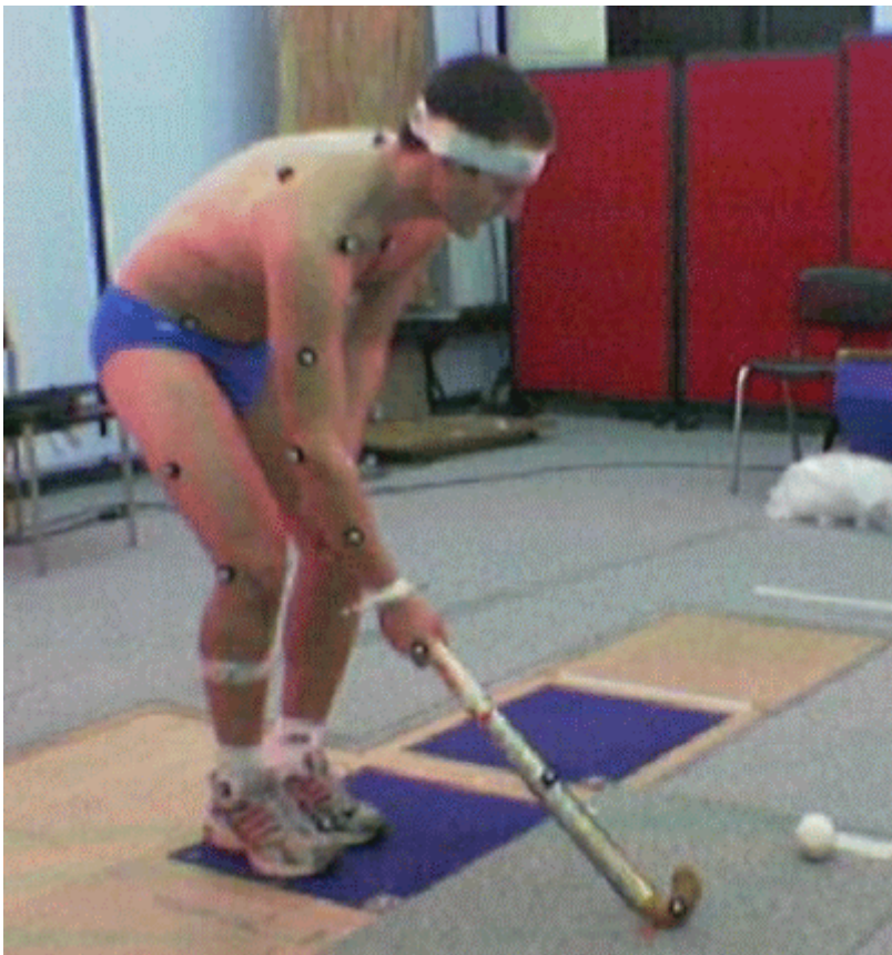
Figure 6 – Starting position and marker set: full body conventional PlugIn Gait on the body, 4 markers on the stick, 3 on the target.
